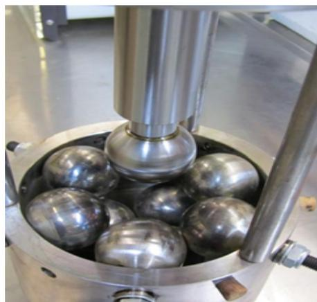
Figure 7: Steel ball assembly
